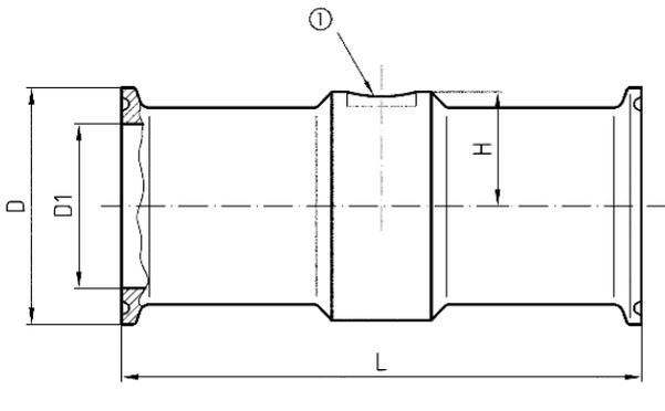
Welded connection  $\varnothing$  10 for measuring instrument
