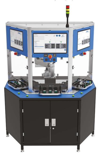
The CRAE - Connector Robotic Assembly Equipment, is a semi-automatic robotic system designed to assembly connector parts.
