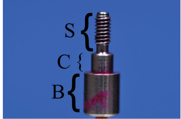
Figure 3 Site evaluation: Body (B) of the abutment represents three sections: implant, mid, occlusal – all showing phloxine B staining and residual contamination. Connection (C) to implant site. Screw (S) thread shank and threads.
