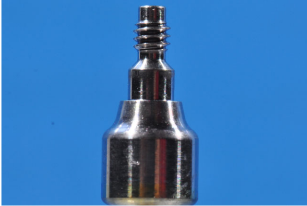
Figure 1 As received specimen, reportedly: Used, wiped, cleaned, and autoclaved.
