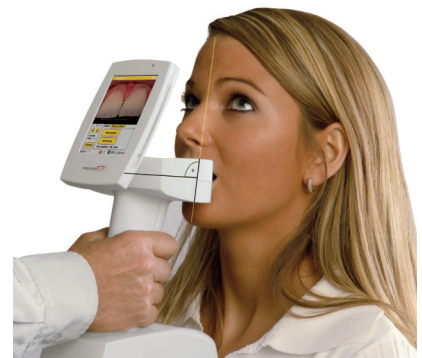
Figure 11. The ShadePilot tooth shade analyzer from DeguDent (Dentsply) features a digital camera linked to a LED spectrophotometer.
