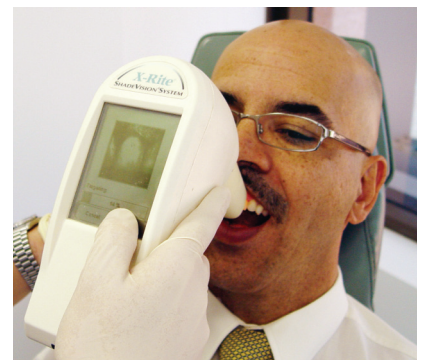
Figure 13. The X-Rite ShadeVision (Henry Schein) incorporates a colourimeter and integrated light source.
