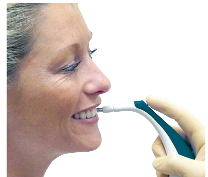
Figure 12. The VITA Easyshade (Henry Schein) integrates a powerful spectrophotometer into a small and compact unit for determining the shades of teeth.
